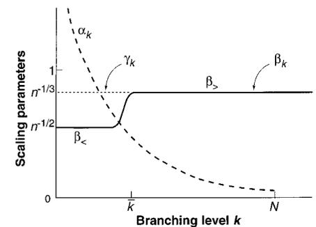
**Fig. 2.** Schematic variation of the Womersley number  $\alpha_k$  and the scaling parameters  $\beta_k$  and  $\gamma_k$  with level number ( $k$ ) for pulsatile systems. Note the steplike change in  $\beta_k$  at  $k = \bar{k}$  from area-preserving pulse-wave flow in major vessels to area-increasing Poiseuille-type flow in small vessels.
